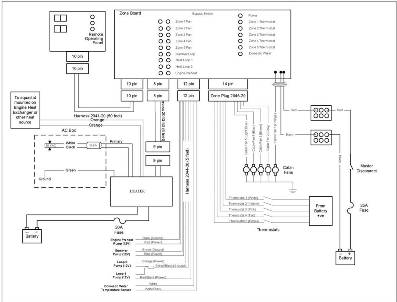
Figure 9-10: Zone Board Wiring (No DM12)
