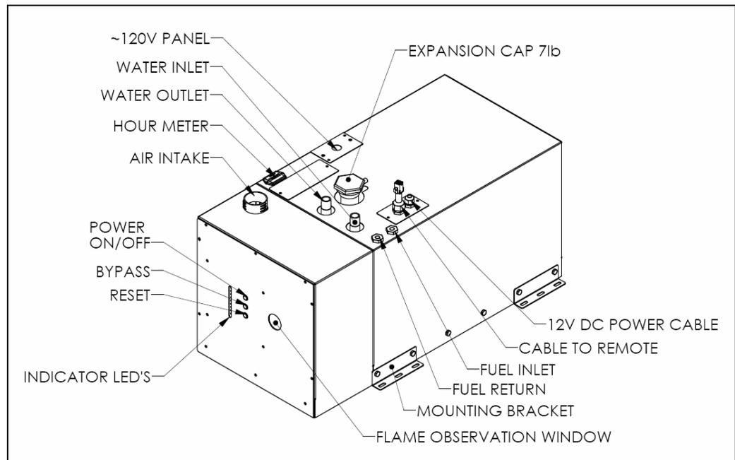
**Figure 7-1 Heating Module**
