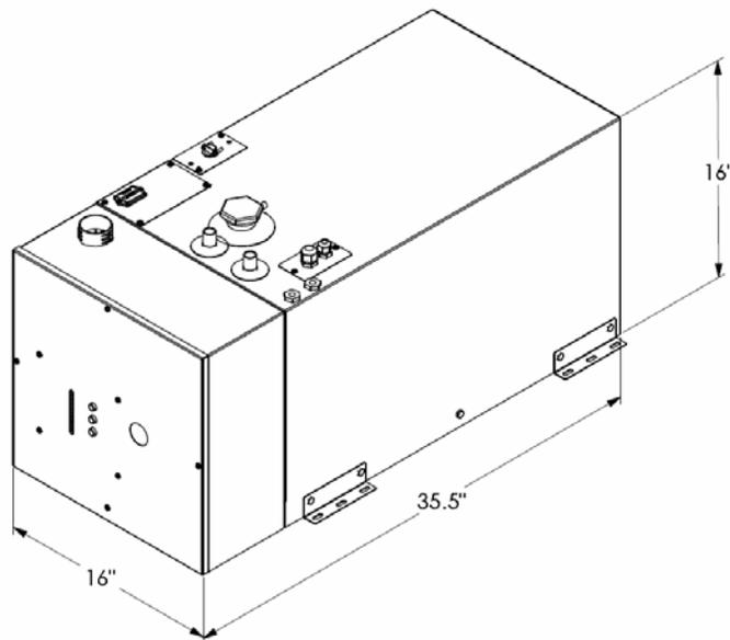
**Figure 2-1: Module Dimensions**
