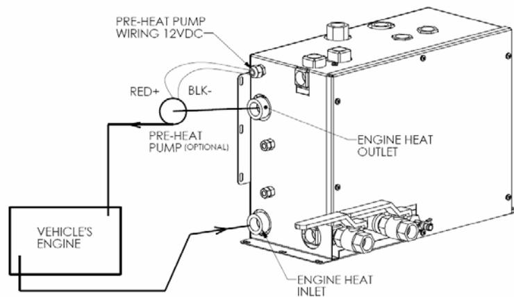
**Figure 9-5 Engine Heat / Pre-heat System Plumbing.**
