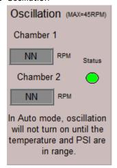
The RPM can be set here or oscillation. And also shows the status. In Auto mode, oscillation will not turn on until the temperature and PSI are in range.
