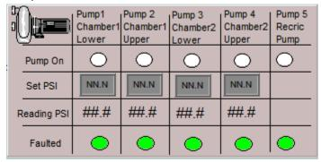
The pump PSI can be set here for auto mode and it shows the pump status.
