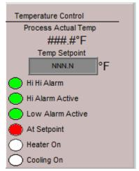
The temp setpoint can be set here. Please see the system config for alarm setting. MIN:50,MAX:150,Ramp Value:0.5
