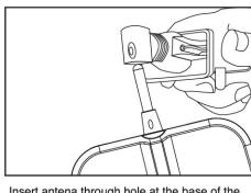
Insert antena through hole at the base of the Smart Phone Mount.
