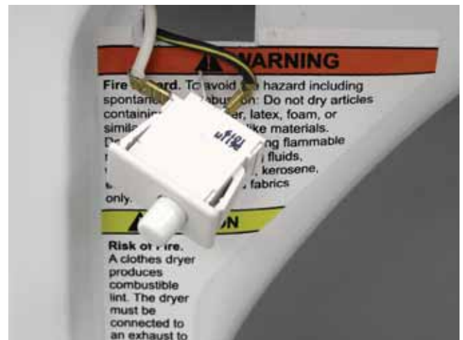
Door Switch (removed)
