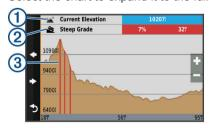
The device displays your current elevation ①, the distance to the next steep grade ②, and a chart of elevation over distance. Steep grades ③ are highlighted red on the chart.
