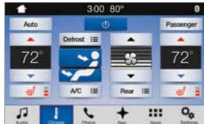
SYNC 3 controls the temperature, airflow direction, fan speed, and activates other climate features, like the heated steering wheel.\* Use the touchscreen to enter into each feature's submenu for additional options.
