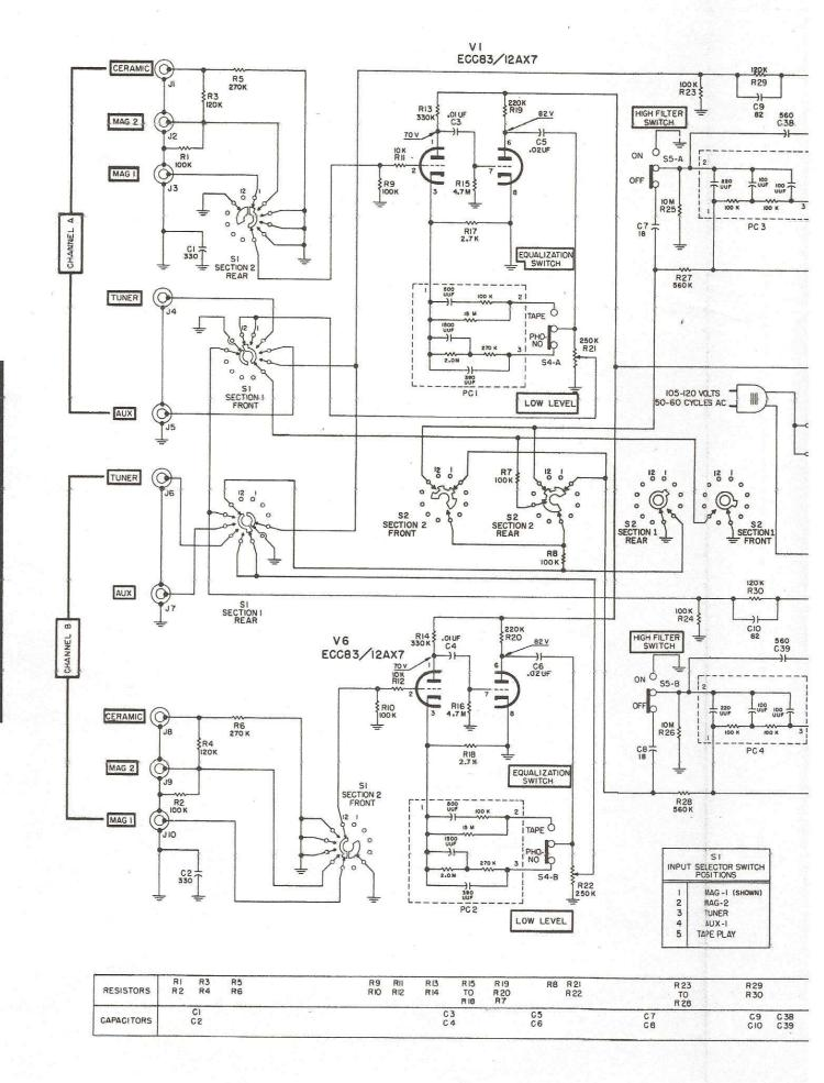
Red lines at C20 and C21 denote schematic errors and are to be disregarded as far as the schematic is concerned. They should NOT be part of the unit. DOUBLE CHECK TO MAKE SURE.
