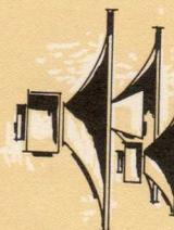
Three-speaker system includes a 15" bass reproducer, 8" mid-range, and an ultra-high-frequency unit for perfect clarity over the entire audible spectrum.
