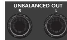
The Mustang Floor provides unbalanced outputs for connection to mono or stereo amplifiers or a combination of sound equipment. Use the utility menu (see Utility Menus, page 7) to adjust the mixing and voicing of the signals sent from these jacks. Use the LEVEL knob to adjust the output level to accommodate the input sensitivity of outboard equipment and avoid unwanted signal distortion.
