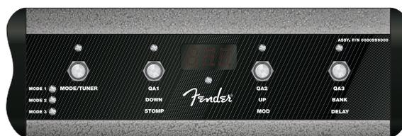
The footswitch has three modes that are identified by the three LEDs labeled **MODE 1**, **MODE 2** and **MODE 3**. The footswitch also has a Tuner mode which is indicated when all of the mode LEDs are off.
