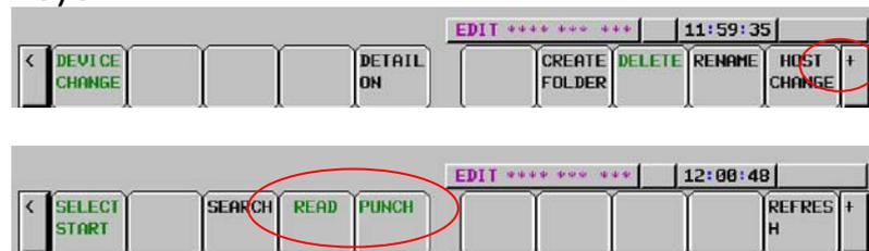
It is important to remember that when you use the Read /Punch function that the files will be transferred to and from the current path set as the Foreground folder.
