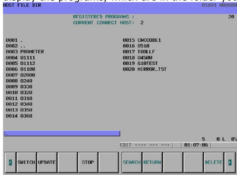
If you press the **▶** soft key you will then see the READ and PUNCH soft keys. If you type 04500 and press the READ soft key, that program will be transferred to the NC memory. If you type a program number that is in the NC memory and press PUNCH it will be transferred to the PC.
