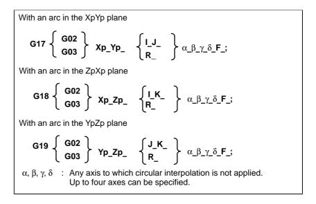
Basically, the command can be specified by adding two movement axes to a standard helical interpolation command (see II–4.5). Address F should be followed by a tangential velocity, which has been determined by also taking movement along the linear axes into consideration.
