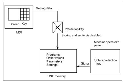
Fig.1.6 (f) Data Protection Key
