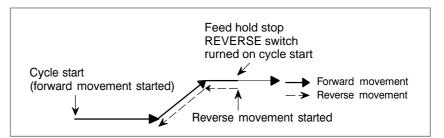
● Reverse movement → Forward return movement Three methods are available for moving the nozzle in the forward direction again along the retraced path.
