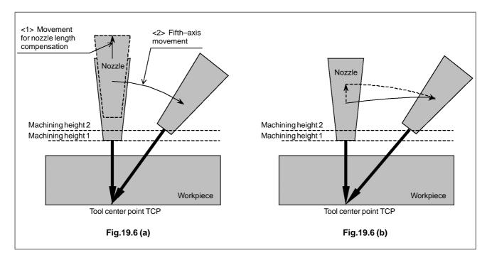
The following shows an example in which the nozzle becomes shorter (the machining height decreases) depending on the machining attitude.
