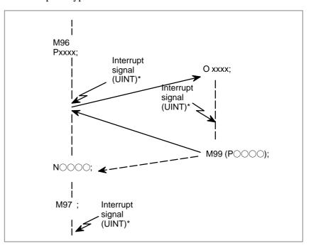
Fig.13.11 Interruption type sustom macro function
