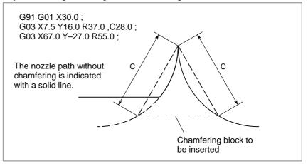
If no arc end point is specified with a G02 or G03 command, the machine tool does not operate properly.
