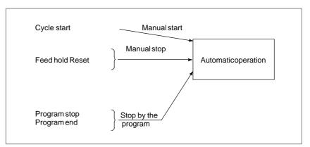
Fig.1.3 (b) Starting and Stopping Automatic Operation
