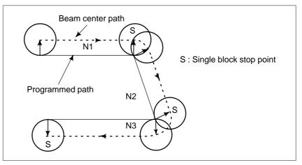
Fig.12.7 (e) Point at which a Single–Block Stop Occurs in the Normal Direction Control Mode
