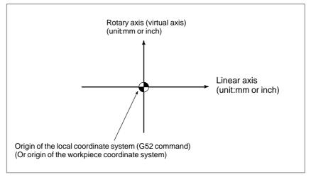
Fig.4.7 Polar coordinate interpolation plane.
