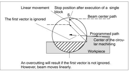
Starting compensation and cutting along the Z–axis It is usually used such a method that the beam is moved along the Z axis after the cutter compensation is effected at some distance from the workpiece at the start of the machining.
