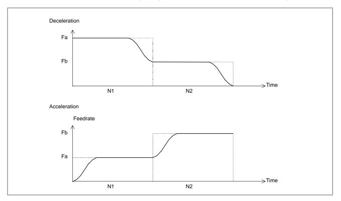
Automatic corner deceleration Between contiguous two blocks, the feedrate difference for an axis may exceed the setting (parameter No. 1783). In this case, the feedrate at the corner is calculated as follows based on the axis for which the ratio of the actual feedrate difference to the allowable feedrate difference is the largest. Deceleration is performed so that the feedrate is reached at the interface of the blocks.
