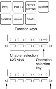
The function keys are used to select the type of screen (function) to be displayed. When a soft key (section select soft key) is pressed immediately after a function key, the screen (section) corresponding to the selected function can be selected.
