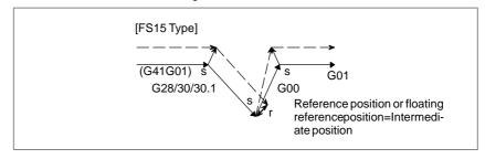
(4)G28, G30, or G30.1 specified in offset mode (with no movement performed)
