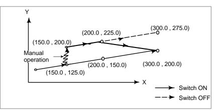
When reset after a manual operation following a feed hold Coordinates when the feed hold button is pressed while block [2] is being executed, manual operation (Y-axis +75.0) is performed, the control unit is reset with the RESET button, and block [2] is read again
