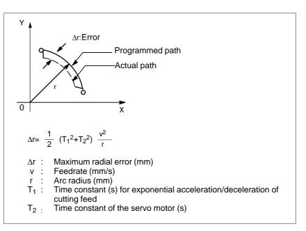
When actual machining is performed, radius r of the arc to be machined and permissible error Dr are given. Then, maximum allowable feedrate v (mm/min) is determined from the above expression.
