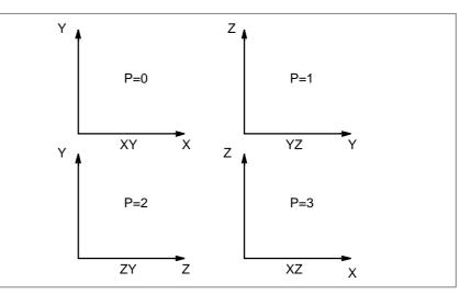
Fig.12.2.1 (a) Coordinate systems for the plane view
