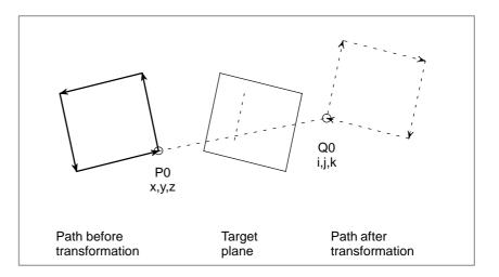
Three–dimensional movement transform When the three base points before transformation, (P1,P2,P3), and the target points after transformation, (Q1,Q2,Q3), are specified, the coordinate system after transformation is obtained. The program to be transformed moves to the coordinate system.
