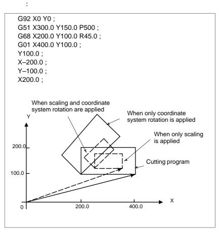
Fig.12.6 (e) Scaling and coordinate system rotation in cutter compensation C mode
