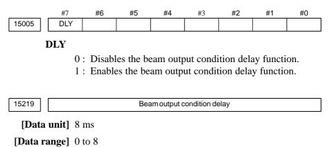
The change of beam output conditions is delayed by the value set for this parameter.
