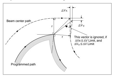
If  $\Delta Vx \leq \Delta V$  limit and  $\Delta Vy \leq \Delta V$  limit, the latter vector is ignored. The  $\Delta V$  limit is set in advance by parameter (No. 5010).
