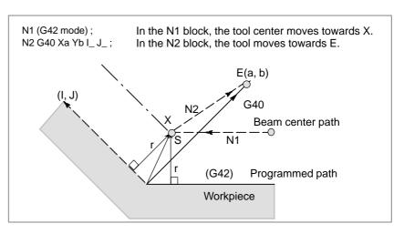
In this case, note that the CNC obtains an intersection of the beam path irrespective of whether inner or outer side machining is specified
