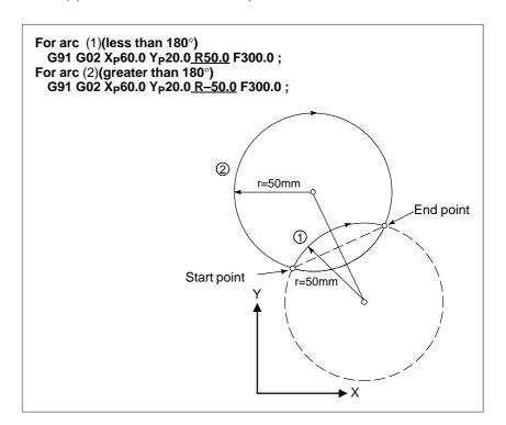
The feedrate in circular interpolation is equal to the feed rate specified by the F code, and the feedrate along the arc (the tangential feedrate of the arc) is controlled to be the specified feedrate.
