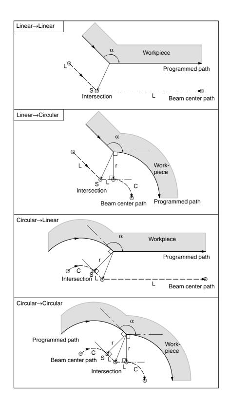
Nozzle movement around the outside corner at an acute angle (α<90°)</li>
