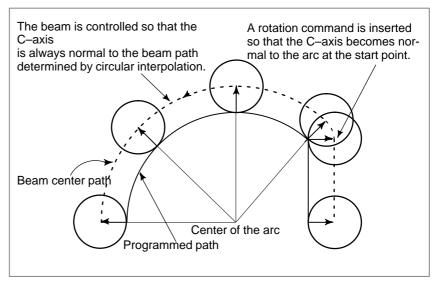
Fig.12.7 (f) Normal direction control of the circular interpolation
