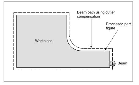
If radius of beam are stored in the CNC (Data Display and Setting : see III–11), the tool can be moved by cutter radius apart from the machining part figure. This function is called cutter compensation (See II–12.2 and 12.3).
