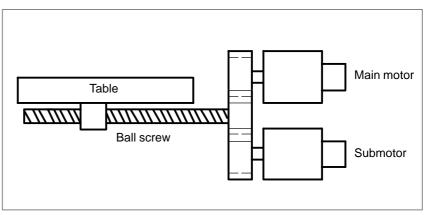
Fig.17.3 Example of operation
