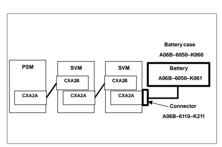
If a low battery voltage or a battery voltage of 0 V is indicated by an APC (absolute pulse coder) alarm, replace the battery.
