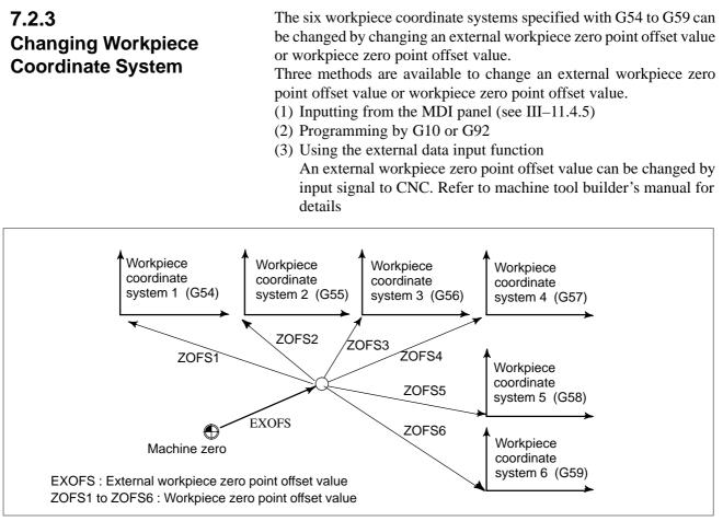
Fig.7.2.3 Changing an external workpiece zero point offset value or workpiece zero point offset value
