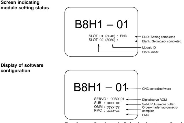
The software configuration can be displayed on the system configuration screen also.
