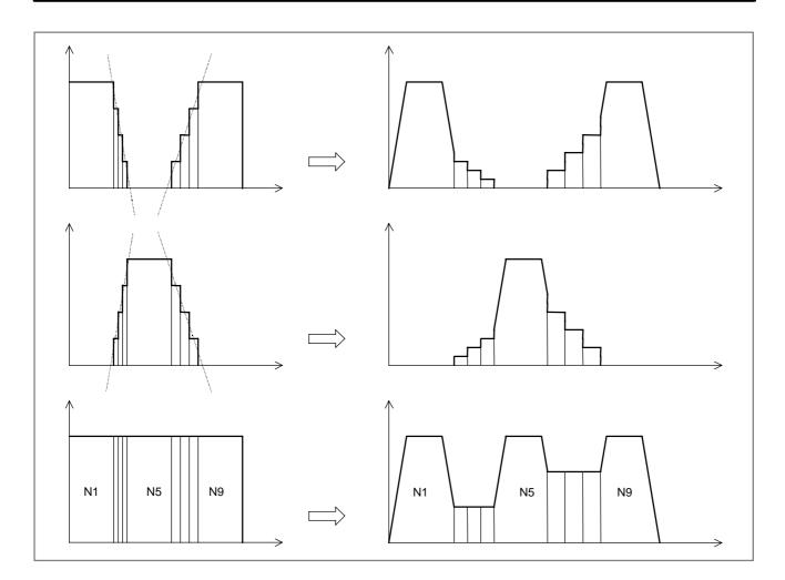
• Feedrate clamping by arc radius
