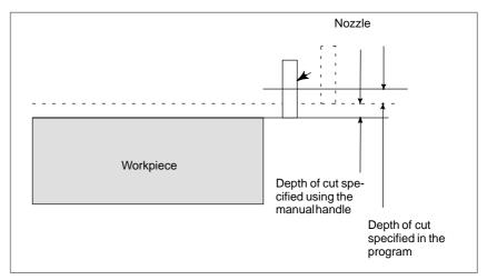
Fig.1.3 (c) Handle Interruption during Automatic Operation
