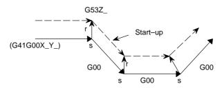
2 When a G53 block is specified to become a start-up block, the next block actually becomes the start-up block. When CCN (bit 2 of parameter No. 5003) is set to 1, an intersection vector is generated.
