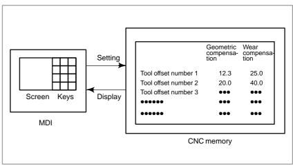
Fig.1.6 (b) Displaying and Setting Offset Values
