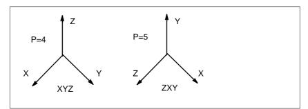
Fig.12.2.1 (b) Coordinate systems for the isometric projection
