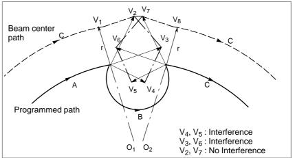
(Example 2) The beam moves linearly from  $V_1$ ,  $V_2$ ,  $V_7$ , to  $V_8$
