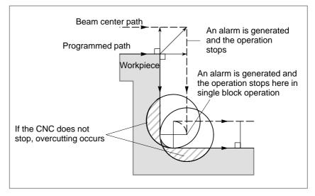
• Machining a groove smaller than the beam radius
