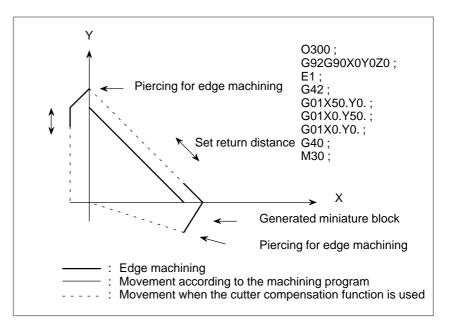
(1) Piercing for edge machining is performed before a miniature block.
