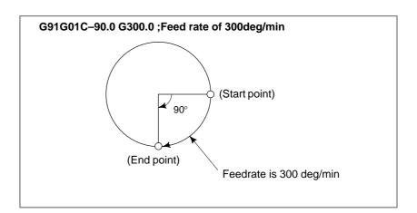
The command below will move a nozzle along a circular arc.
