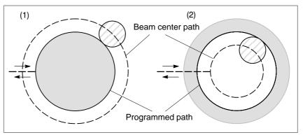
Fig.12.2 (d) Beam Center Paths when Positive and Negative Cutter Compensation Values are Specified
