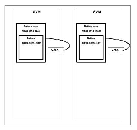
If a low battery voltage or a battery voltage of 0 V is indicated by an APC (absolute pulse coder) alarm, replace the battery(A06B–6073–K001).
