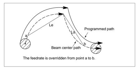
Fig.5.4.2.1 (c) Override Range (Arc to Arc)
