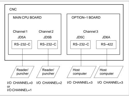
CNC has three channels of reader/punch interfaces. The input/output device to be used is specified by setting the channel connected to that device in setting parameter I/O CHANNEL.
