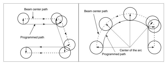
Fig.12.7 (b) Normal direction control left (G41.1)
