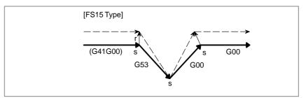
(2) Incremental G53 specified in offset mode When CCN (bit 2 of parameter No.5003)=0
