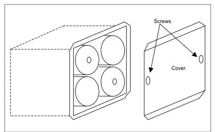
• Attach the lithium battery to the amplifier. (Method 2) Attach the lithium (A06B–6093–K001) battery to the amplifier. [Attachment procedure]
