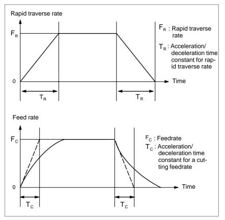
Fig.5.1 (a) Automatic acceleration/deceleration (example)
