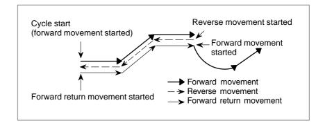
● Reverse movement → Reverse movement completion → Forward return movement If the beam moves in the reverse direction after a feed hold stop, the beam stops forward return movement at the position of the feed hold stop, then resumes forward movement. If the beam moves in the reverse direction after a single block stop, the nozzle also stops forward return movement at the position of the single block stop.
