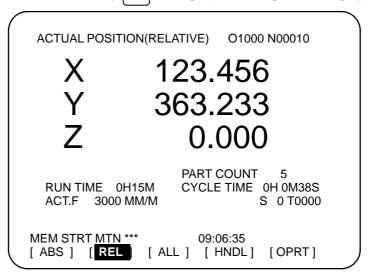
The number of machined parts (PART COUNT), run time (RUN TIME), and cycle time (CYCLE TIME) are displayed under the current position.
