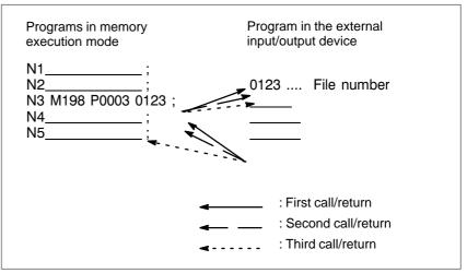
Fig.4.7 Program Flow When M198 is Specified
