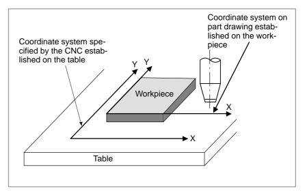
The positional relation between these two coordinate systems is determined when a workpiece is set on the table.
