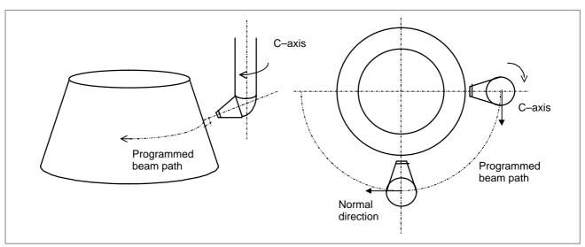
Fig.12.7 (a) Nozzle Operation (Example)
