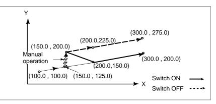
When a movement command in the next block is only one axis When there is only one axis in the following command, only the commanded axis returns.
