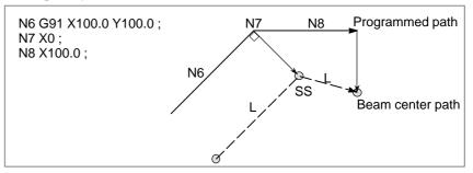
Two blocks without beam movement should not be commanded consecutively. If commanded, a vector whose length is equal to the offset value is produced in a normal direction to beam motion in earlier block, so overcutting may result.
