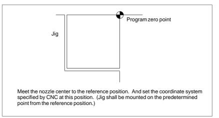
(3) Mounting a workpiece on a pallet, then mounting the workpiece and pallet on the jig
