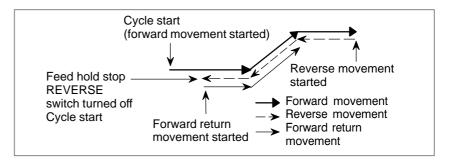
When there are no more blocks for which to perform reverse movement (when the nozzle has moved back to the initial forward movement block or the nozzle has not yet started forward movement), the reverse movement completion state is entered and operation stops.
