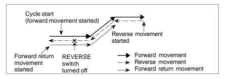
In the case of 2) above, the nozzle starts forward return movement at the position of a single block stop when the cycle start switch is pressed.
