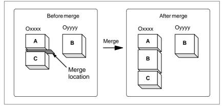
Fig.9.6.4 Merging a program at a specified location
