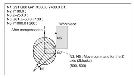
As the block with sequence No. N2 has the move command in the same direction as that of the block with sequence No. N6, the correct compensation is performed.
