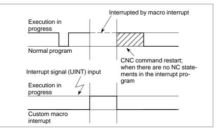
Type II (when an interrupt is performed at the end of the block) (i) If the block being executed is not a block that consists of several cycle operations such as automatic reference position return (G28), an interrupt is performed as follows:When an interrupt signal (UINT) is input, macro statements in the
