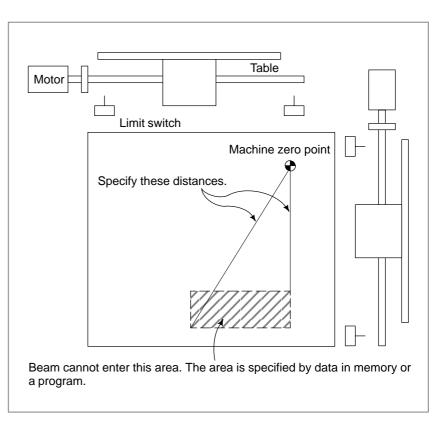
Besides strokes defined with limit switches, the operator can define an area which the nozzle cannot enter using a program or data in memory. This function is called stroke check (see III–6.3).
