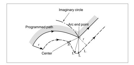
• When the offset mode is canceled temporarily In the HPCC mode, automatic reference position return (G28) and automatic return from the reference position (G29) cannot be specified. Therefore, commands that must cancel the offset mode temporarily cannot be specified.
