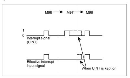
The interrupt signal (UINT) becomes valid after M96 is specified. Even when the signal is input in M97 mode, it is ignored. When the signal input in M97 mode is kept on until M96 is specified, a custom macro interrupt is initiated as soon as M96 is specified (only when the status–triggered scheme is employed); when the edge–triggered scheme is employed, the custom macro interrupt is not initiated even when M96 is specified.
