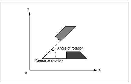
Fig.12.6 (a) Coordinate system rotation
