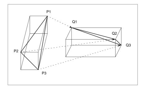
Specifying mirror image transform and movement transform simultaneously Mirror image transform and movement transform can be specified simultaneously.
