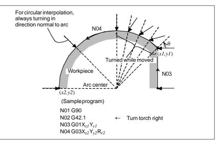
Fig. 19.10 (c) Turning the torch right
