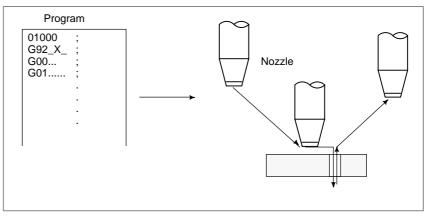
Fig.1.2 (a) Moving the Nozzle Using a Program
