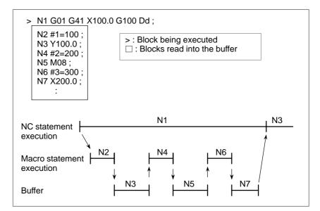
When the NC1 block is being executed, the NC statements in the next two blocks (up to N5) are read into the buffer. Since N5 is a block that involves no movement, an intersection cannot be calculated. In this case, the NC statements in the next three blocks (up to N7) are read. The macro statements (N2, N4, and N6) between N1 and N7 are processed during execution of N1.
