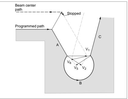
After ignoring vectors  $V_2$  and  $V_5$  because of interference, interference also occurs between vectors  $V_1$  and  $V_6$ . The alarm is displayed and the beam is stopped.
