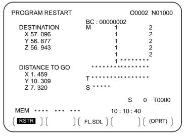
DESTINATION indicates the position at which processing is to restart.
