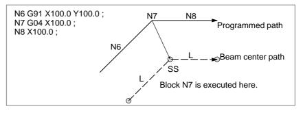
However, when the move distance is zero, even if the block is commanded singly, beam motion becomes the same as that when more than one block of without beam movement are commanded, which will be described subsequently.
