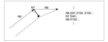
If cutter compensation mode is canceled while a vector still remains and HPCC mode is canceled before a move command is specified, the P/S alarm No.5013 is issued.
