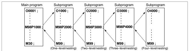
A single call command can repeatedly call a subprogram up to 999 times. For compatibility with automatic programming systems, in the first block, Nxxxx can be used instead of a subprogram number that follows O(or:). A sequence number after N is registered as a subprogram number. PROGRAMMING
