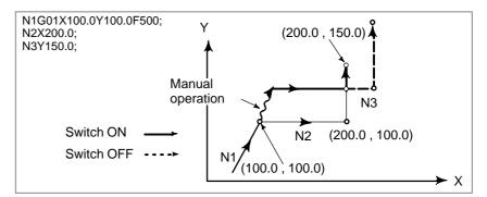
When the next move block is an incremental When the following commands are incremental commands, operation is the same as when the switch is OFF.
