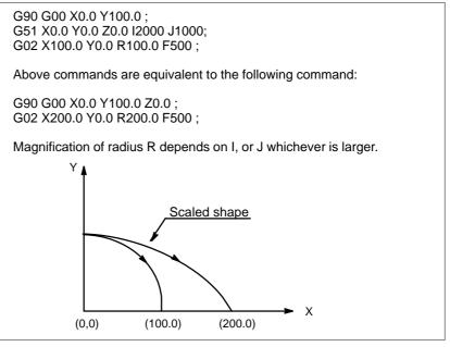
Fig.12.5 (c) Scaling for circular interpolation1
