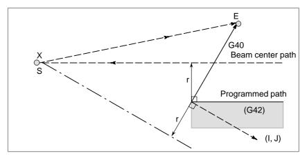
When an intersection is not obtainable, the beam comes to the normal position to the previous block at the end of the previous block.
