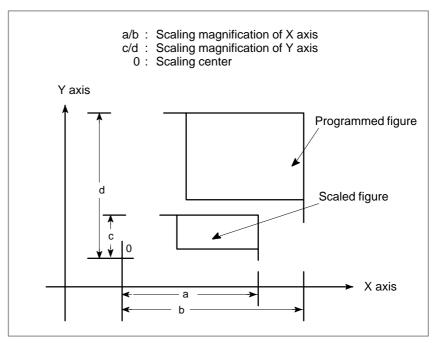
Fig.12.5 (b) Scaling of each axis
