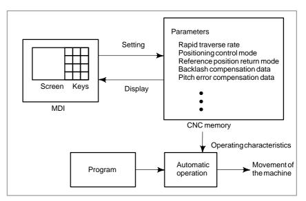
Fig.1.6 (e) Displaying and Setting Parameters
