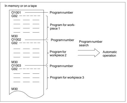
Fig.1.3 (a) Selecting a Program for Automatic Operation
