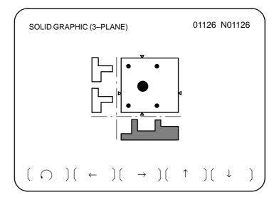
17 Each time soft key [ ) is pressed, the side–view drawings displayed change as follows.
