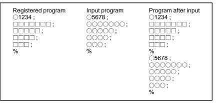
In the above example, all lines of program O5678 are appended to the end of program O1234. In this case, program number O5678 is not registered. When inputting a program to be appended to a registered program, press the **[READ]** soft key without specifying a program number in step 8. Then, press the **[CHAIN]** and **[EXEC]** soft keys.
