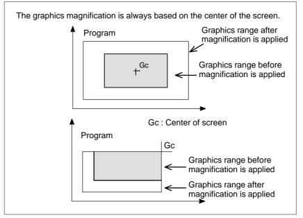
Fig.12.1 (b) Applying graphics magnification (Example of enlargement)
