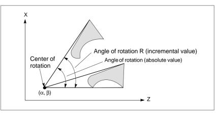
Fig.12.6 (b) Coordinate system rotation
