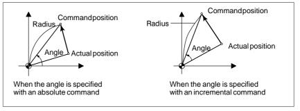
Setting the current position as the origin of the polar coordinate system Specify the radius (the distance between the current position and the point) to be programmed with an incremental command. The current position is set as the origin of the polar coordinate system.
