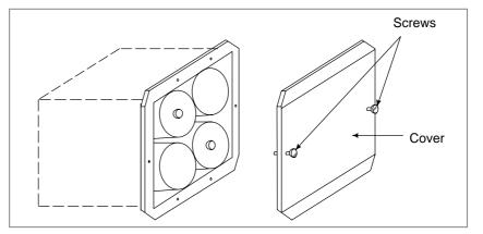
(4) After installing the new batteries, replace the cover.(5) Turn off the power to the machine (*i* Series CNC).
