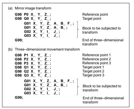
When the program is executed, the coordinates at the base and target points are written into the settings. When Q0 or Q3 is read, transform processing starts according to the values of the settings.
