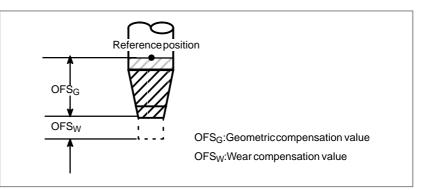
Fig.12.4 (a) Geometric compensation and wear compensation
