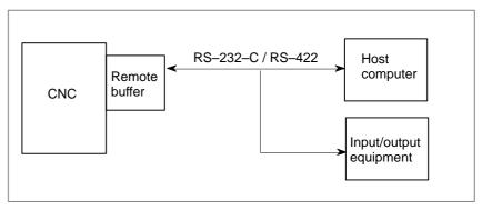
When the remote buffer is connected online to the host computer, fast and reliable DNC operation is possible.
