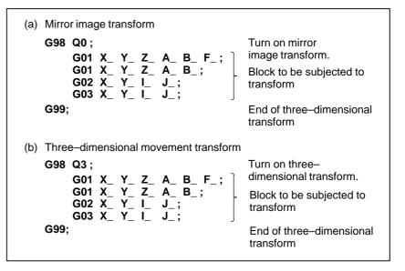
Set the coordinates at the base and target points on the setting screen (see Part III, "Operation") in advance and specify the above command in the program.
