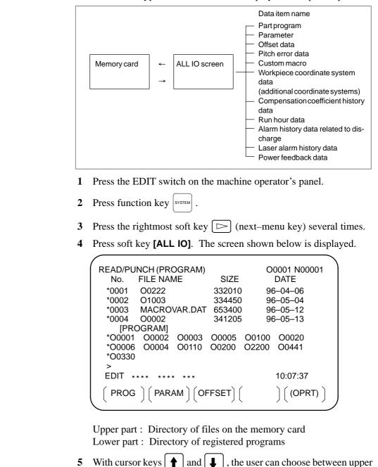
part scrolling and lower part scrolling. (An asterisk (\*) displayed at the left edge indicates the part for which scrolling is possible.)
