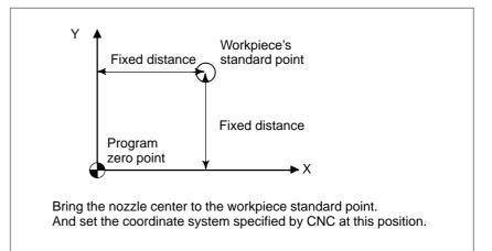
Methods of setting the two coordinate systems in the same position (2) Mounting a workpiece directly against the jig
