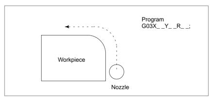
Fig.1.1 (b) Nozzle movement along an arc
