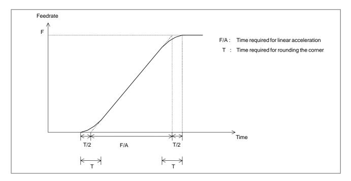
When the non-linear interpolation type is selected, movement is performed at the feedrate set in parameter No. 1420 with acceleration/deceleration set in parameter No. 1620. The corresponding value can be set in parameter No. 1621 to select bell-shaped acceleration/deceleration. (To select bell-shaped acceleration/deceleration, the option of bell-shaped acceleration/deceleration/deceleration for rapid traverse is required.)
