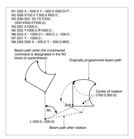
Fig.12.6 (c) Absolute/incremental command during coordinate system rotation
