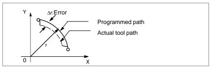
Fig.5.1 (c) Example of Radial Error in Circular Interpolation
