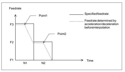
To decelerate from feedrate F3 to F2, deceleration must start with point 1. To decelerate from feedrate F2 to F1, deceleration must start with point 2.
