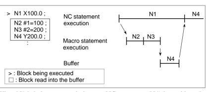
When N1 is being executed, the next NC statement (N4) is read into the buffer. The macro statements (N2, N3) between N1 and N4 are processed during execution of N1.
