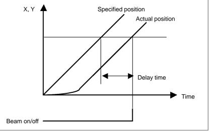
Conceptual diagram of beam delay control
