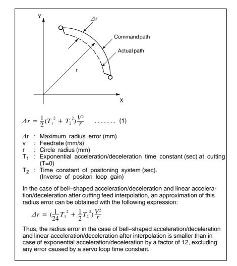
Since the machining radius r (mm) and allowable error  $\Delta r$  (mm) of the workpiece is given in actual machining, the allowable limit feedrate (mm/sec) is determined by equation (1).
