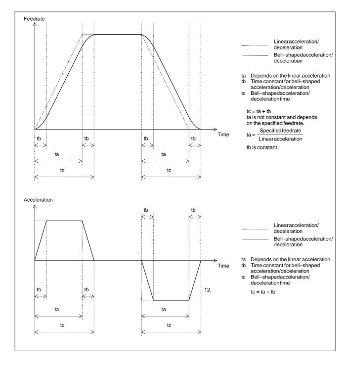
When the feedrate is changed, deceleration and acceleration are performed as follows:
