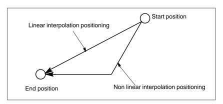
The rapid traverse rate in G00 command is set to the parameter No. 1420 for each axis independently by the machine tool builder. In the posiitoning mode actuated by G00, the tool is accelerated to a predetermined speed at the start of a block and is decelerated at the end of a block. Execution proceeds to the next block after confirming the in–position.
