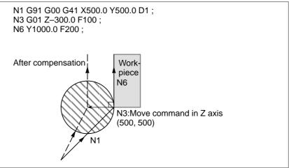
In the program example above, when executing block N1, blocks N3 and N6 are also entered into the buffer storage, and by the relationship among them the correct compensation is performed as in the figure above.
