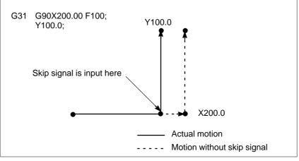
Fig.4.10 (b) The next block is an absolute command for 1 axis
