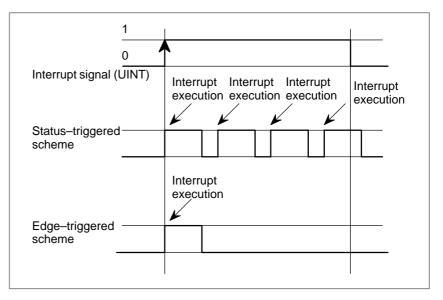
In the above example, an interrupt is executed four times when the status triggered scheme is used; when the edge– triggered scheme is used, the interrupt is executed just once.
