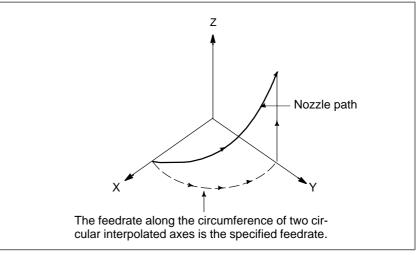
•Cutter compensation is applied only for a circular arc. •Tool offset and tool length compensation cannot be used in a block in which a helical interpolation is commanded.
