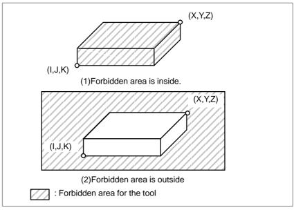
Fig.6.3 (a) Stroke check
