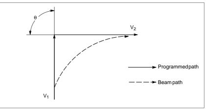
Fig.D.1 (a) Slight deviation between the beam path and the programmed path
