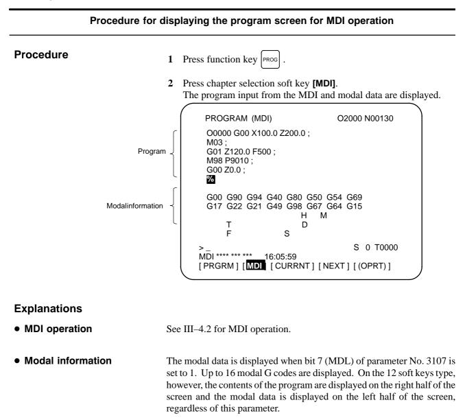
• Displaying during automatic operation During automatic operation, the actual speed, SACT, and repeat count are displayed. The key input prompt (>\_) is displayed otherwise.
