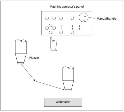
Fig.1.1 (b) Moving the Nozzle Manually
