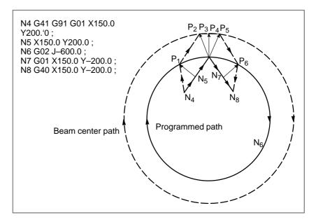
If the vector is not ignored, the beam path is as follows:  $P_1 \rightarrow P_2 \rightarrow P_3 \rightarrow (Circle) \rightarrow P_4 \rightarrow P_5 \rightarrow P_6$ But if the distance between P2 and P3 is negligible, the point P3 is ignored. Therefore, the beam path is as follows:  $P_2 \rightarrow P_4$ Namely, circle cutting by the block N6 is ignored.
