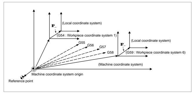
Fig.7.3 Setting the local coordinate system
