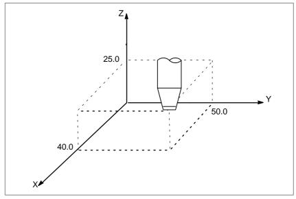
Fig.7 Nozzle position specified by X40.0Y50.0Z25.0
