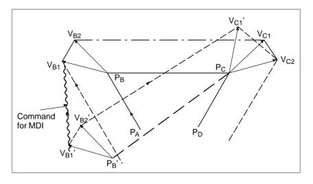
When position  $P_A$ ,  $P_B$ , and  $P_C$  are programmed in an absolute command, beam is stopped by the single block function after executing the block from  $P_A$  to  $P_B$  and the beam is moved by MDI operation. Vectors  $V_{B1}$  and  $V_{B2}$  are translated to  $V_{B1}$ ' and  $V_{B2}$ ' and offset vectors are recalculated for the vectors  $V_{C1}$  and  $V_{C2}$  between block  $P_B$ – $P_C$  and  $P_C$ – $P_D$ .
