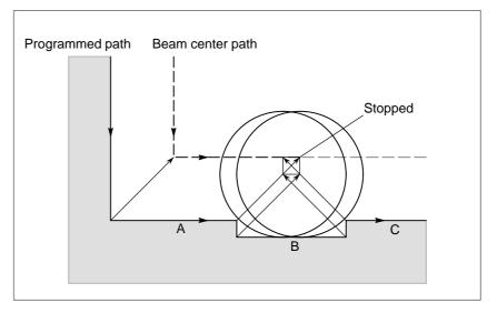
There is no actual interference, but since the direction programmed in block B is opposite to that of the path after cutter compensation the beam stops and an alarm is displayed.
