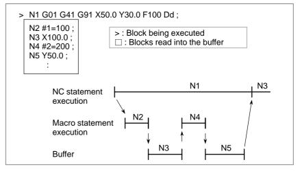
When N1 is being executed, the NC statements in the next two blocks (up to N5) are read into the buffer. The macro statements (N2, N4) between N1 and N5 are processed during execution of N1.
