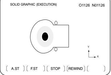
10 Press soft key [(OPRT)] and press either soft key [A.ST] or [F.ST]. When [A.ST] is pressed, the status of machining in progress is drawn by simulation. When [F.ST] is pressed, the profile during machining is not drawn. Only the finished profile produced by the program is drawn. This allows drawing to be started. When "STOP" is not displayed at the lower right corner of the screen, the program is executed from its head. "DRAWING" blinks at the lower right corner of CRT screen during drawing.
