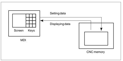
Fig.1.6 (a) Displaying and Setting Data
