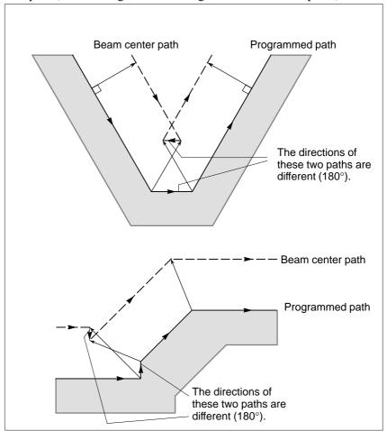
(2) In addition to the condition (1), the angle between the start point and end point on the beam center path is quite different from that between the start point and end point on the programmed path in circular machining(more than 180 degrees).
