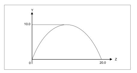
N001 G07 X0 ; N002 G91 G17 G03 X-20.2 Y0.0 I-10.0 Z20.0 F100 ; N003 G01 X10.0 ; N004 G07 X1 ; From the N002 to N003 blocks, the X-axis is set to a hypothetical axis. The N002 block specifies helical cutting in which the Z-axis is the linear
