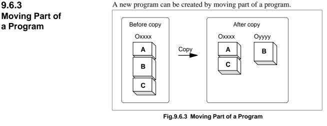
In **Fig.9.6.3**, part B of the program with program number xxxx is moved to a newly created program with program number yyyy; part B is deleted from the program with program number xxxx.
