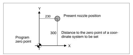
Fig.1.3.2 (b) Coordinate system specified by the CNC
