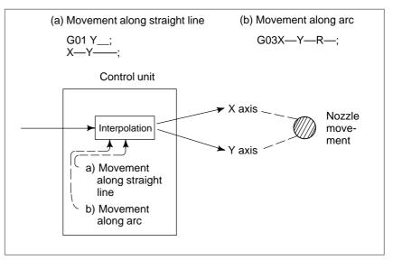
Fig.1.1 (c) Interpolation function
