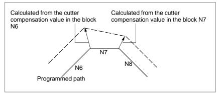
Fig.12.2 (c) Changing the Cutter Compensation Value
