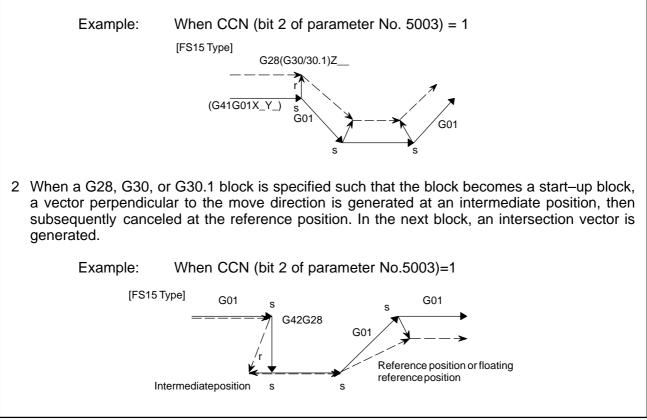
• G29 command in cutter compensation C mode FS15 type is performed if CCN (bit 2 of parameter No. 5003) is set to 1.
