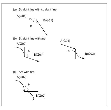
If a calculated angle is smaller than a set value, a corner is assumed; a gradual stop occurs at the end point of block A, and feedrate and power control is applied.
