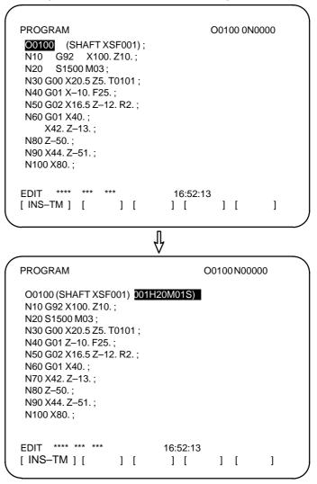
**5** The machining time of a program inserted as a comment can be displayed after an existing program comment on the program directory screen.
