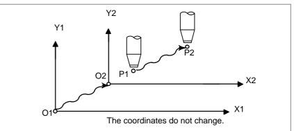
Fig.3.5 (b) Coordinates with the switch OFF
