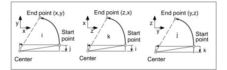
I0,J0, and K0 can be omitted. When  $X_p$ ,  $Y_p$ , and  $Z_p$  are omitted (the end point is the same as the start point) and the center is specified with I, J, and K, a 360° arc (circle) is specified.
