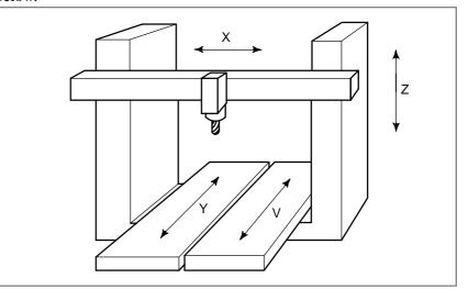
Fig.17.1 Example of axis configuration of the machine operated by simple synchronous control
