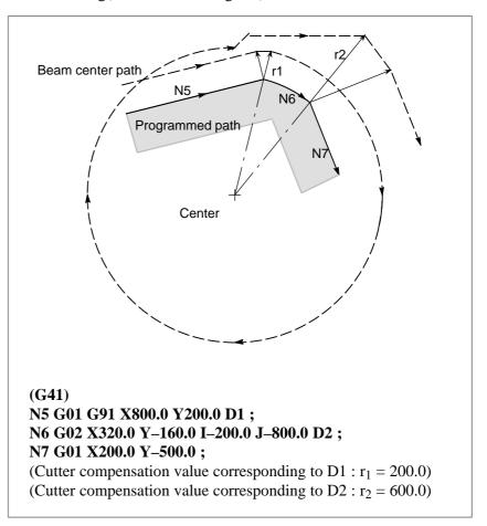
In the above example, the arc in block N6 is placed in the one quadrant. But after cutter compensation, the arc is placed in the four quadrants.
