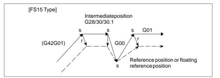
(2) G28, G30, or G30.1, specified in offset mode (with movement to an intermediate position not performed)
