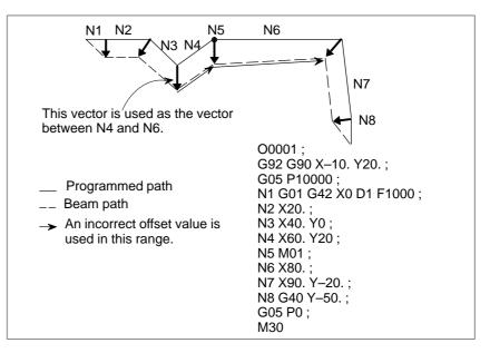
(Example 2) When the following program is executed for machining with offset value D1 set to 10 mm, the start point of N5 is determined by the vector created between N3 and N4. If the simplified G00 execution function is enabled (by setting bit 7 of parameter SG0 No. 8403 to 1), a correct vector can be obtained at the intersection of N4 and N5.
