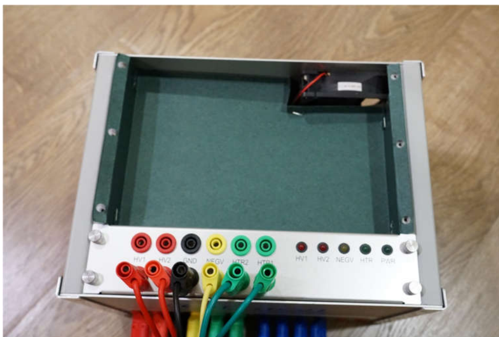
Catch-box installed on the Model-01 chassis
