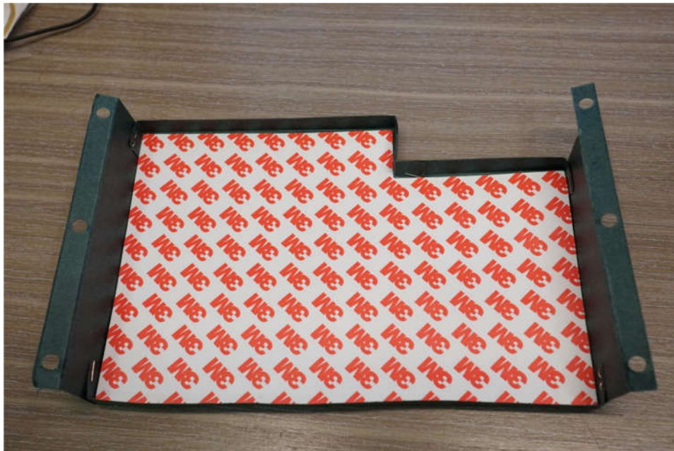
Built catch-box with 3M double-sided tape installed
