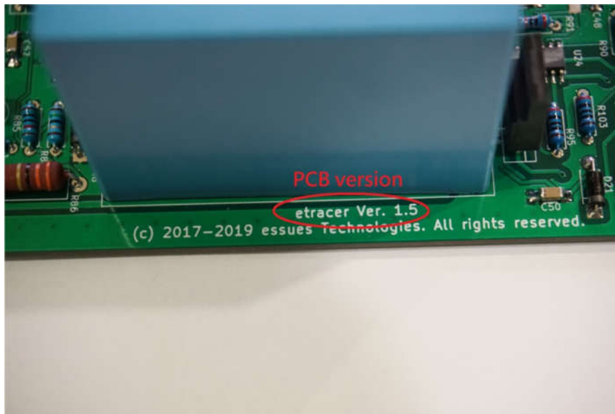
Location of PCB version information on the etracer PCB
