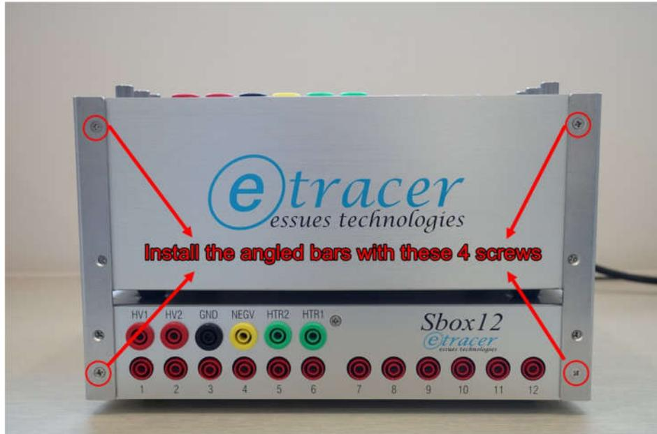
Figure 10. Recommended method to mount the angled bars (2)
