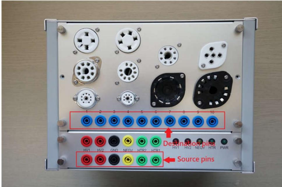
Figure 2. Source pins and destinations pins for the etracer
