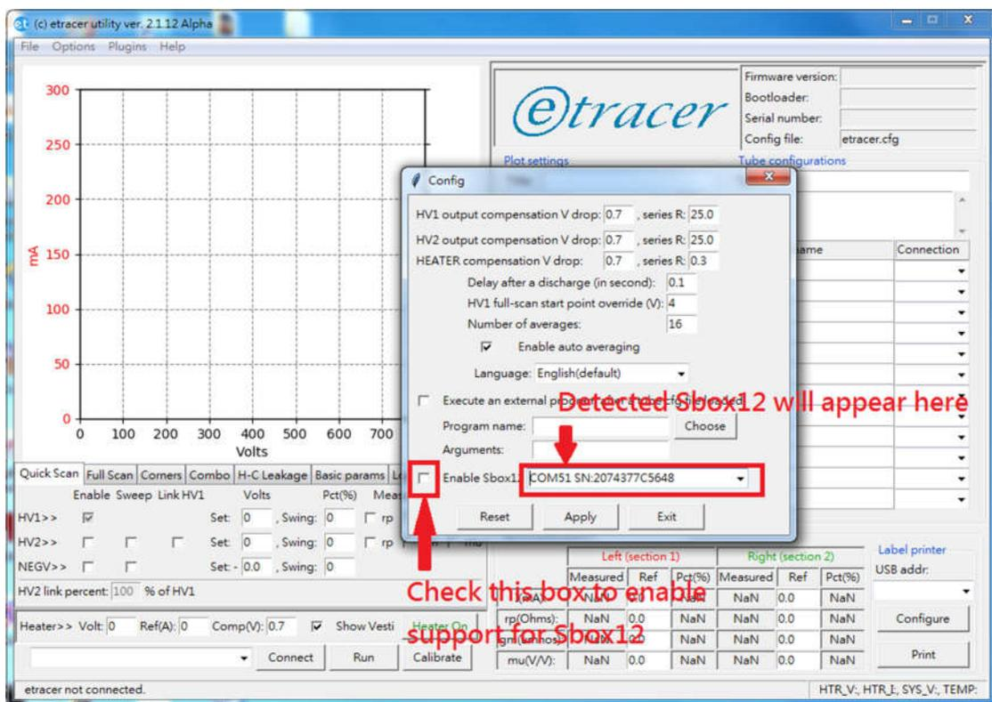
Figure 15. Configure Sbox12 in the configuration window
