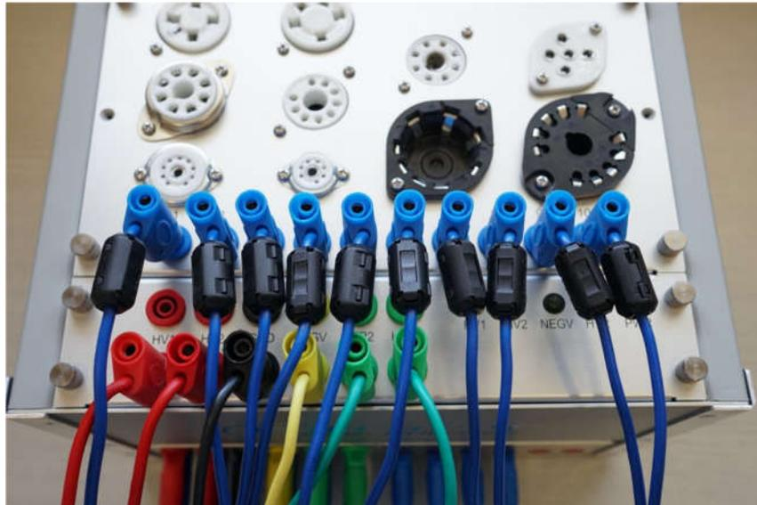
Figure 14. Top view of the wiring for the destination pins.
