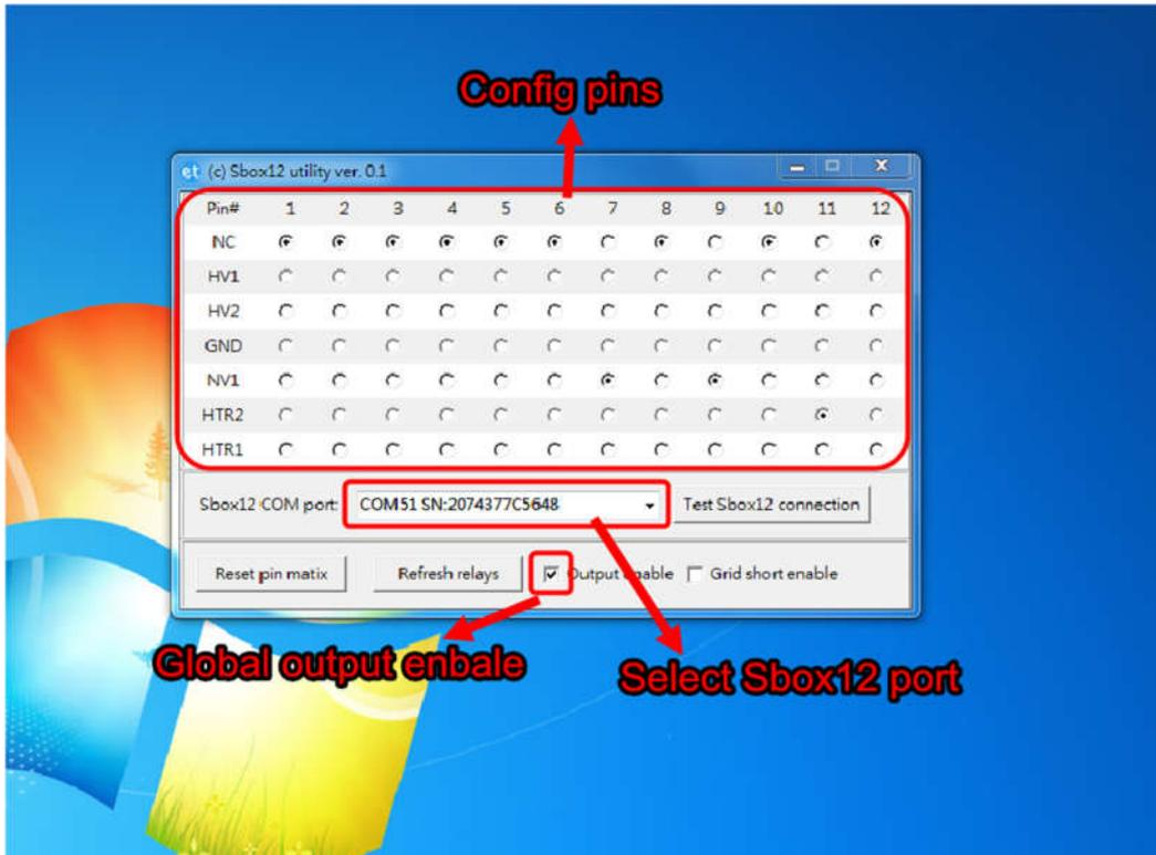
Figure 15. Sbox12 GUI control utility
