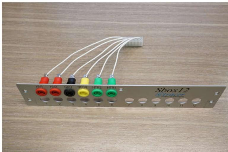
Figure 8. Banana jacks for the source pins and the connecting wires
