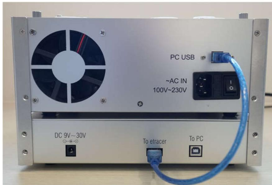
Figure 11. Connection of between etracer and Sbox12.
