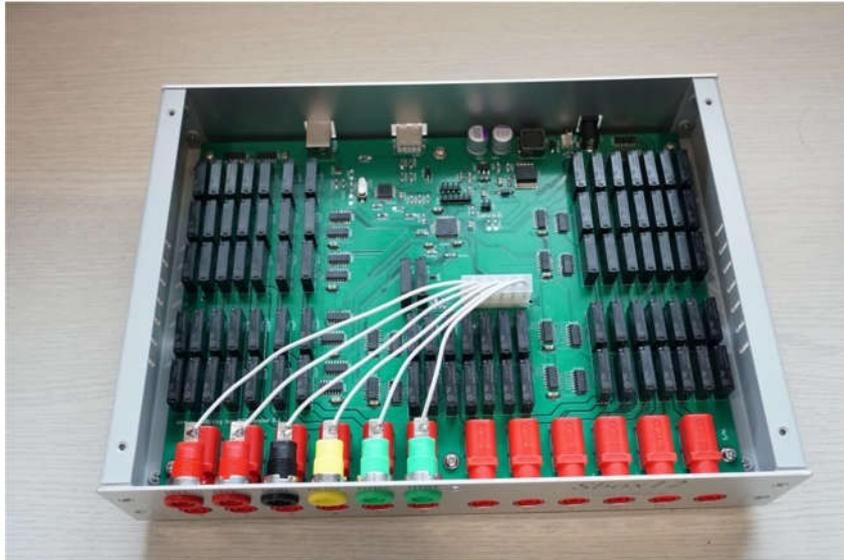
Figure 5. Connecting J114 to the banana jacks on the front panel.
