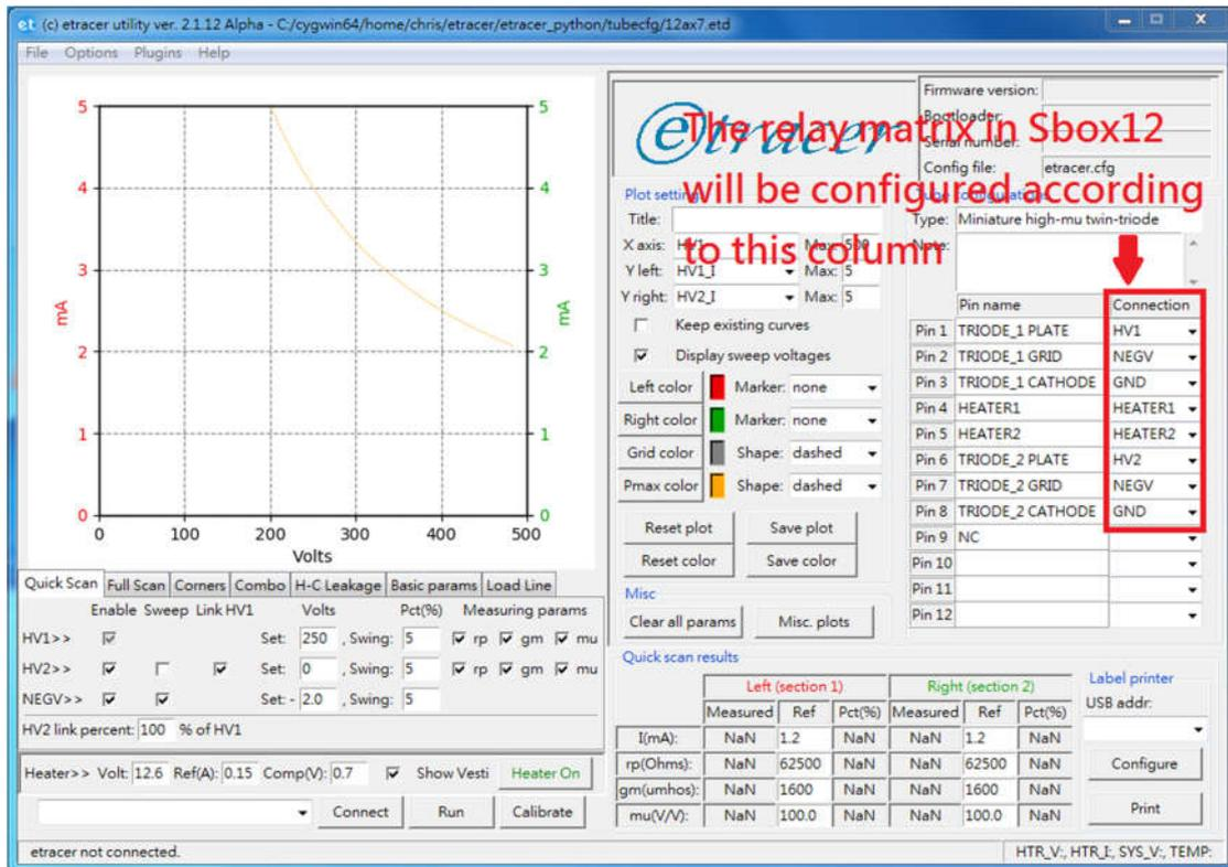
Figure 16. The Sbox12 relay matrix configuration (12AX7 as an example)
