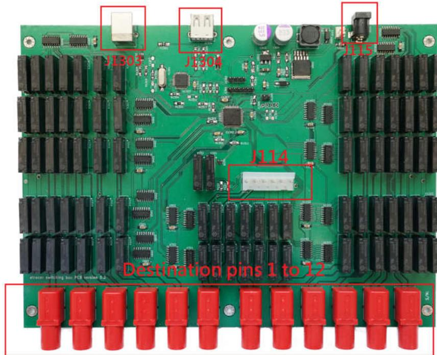
Figure 4. The Sbox12 PCB
