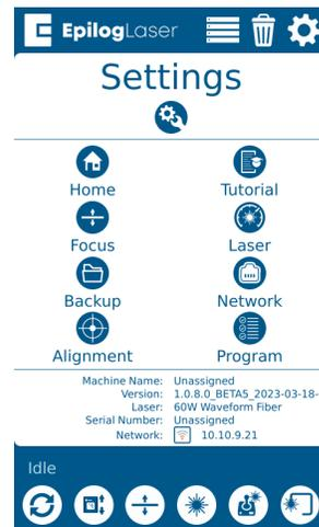
11. Press the Focus button to enter the Focus Command/Calibrations Menu:
