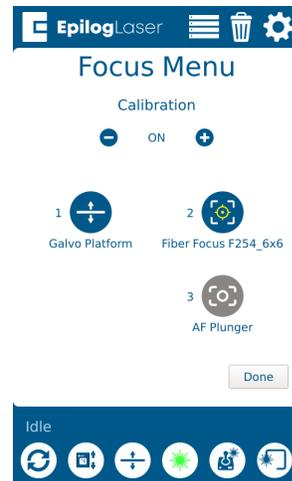
5. Press the Start button to start the Galvo Platform calibration:
