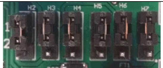
Figure 10. Input/output selection jumpers.
