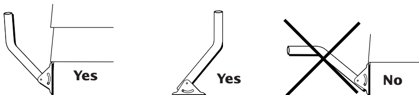
Step 7: Make sure that the top of the mast will point straight up.
