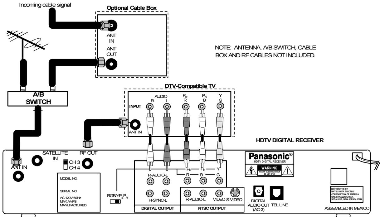
**HDTV DIGITAL RECEIVER WITH DTV-COMPATIBLE TV WITH CABLE SERVICE AND TERRESTRIAL ANTENNA**
