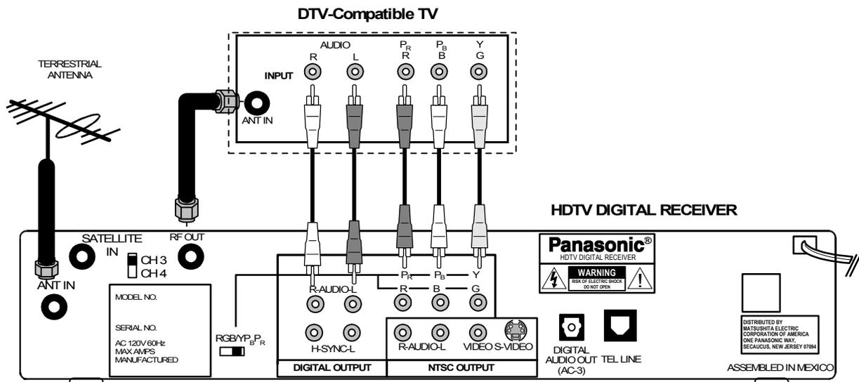
**HDTV DIGITAL RECEIVER, DTV COMPATIBLE TV/MONITOR
