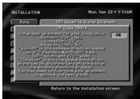
The Alignment Result pop-up panel.
