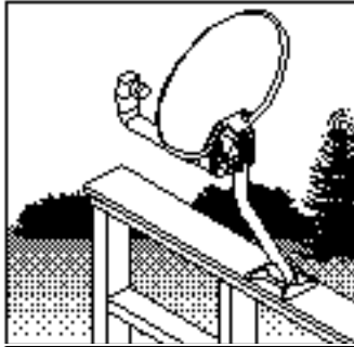
Installing the satellite dish antenna on the rail or floor of a deck. See the section titled "Installing the Satellite Dish Antenna Onto a Wooden Surface."
