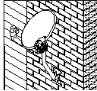
Installing the satellite dish antenna on a brick surface. See the section titled "Installing the Satellite Dish Antenna Onto a Brick Surface."
