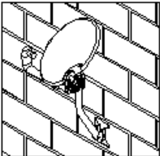
Installing the satellite dish antenna on a cinder block or masonry surface. See the section titled "Installing the Satellite Dish Antenna Onto a Cinder Block Surface."
