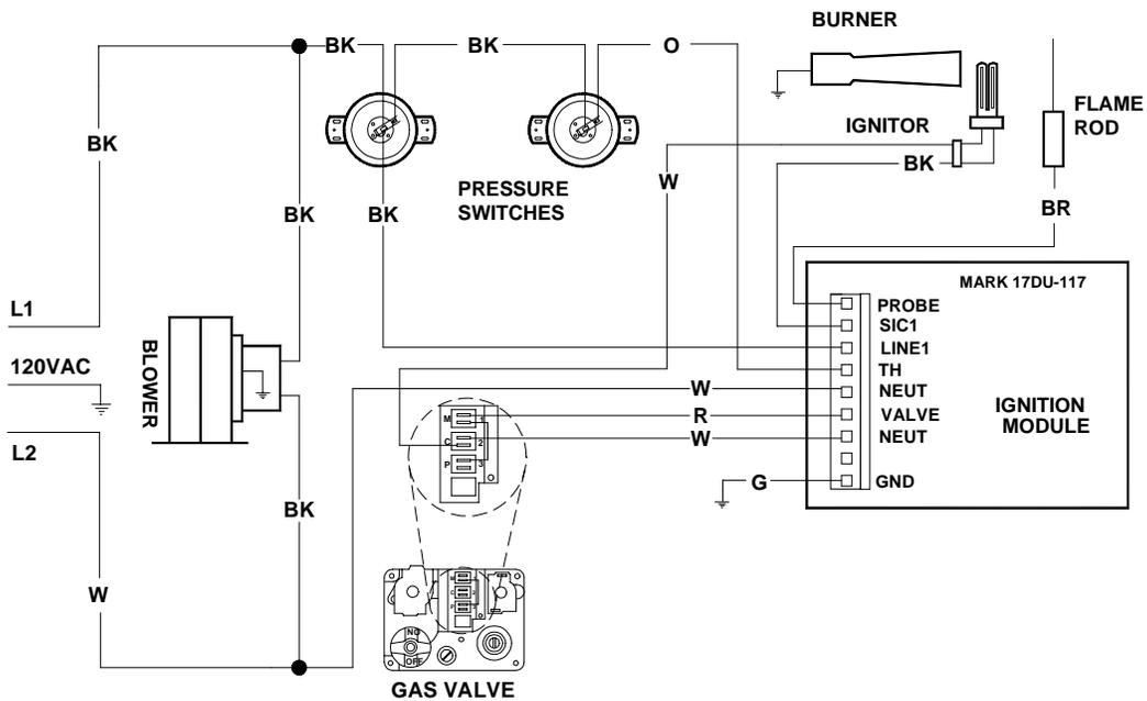
If any of the original wire as supplied with the appliance must be replaced, it must be replaced with wiring material having a temperature rating of at least 105°C.
