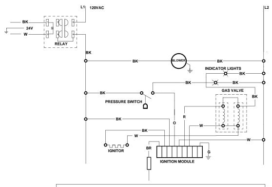
IF ANY OF THE ORIGINAL WIRE AS SUPPLIED WITH THE APPLIANCE MUST BE REPLACED, IT MUST BE REPLACED WITH WIRING MATERIAL HAVING A TEMPERATURE RATING OF AT LEAST 105 C.
