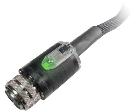
A Smart-Light mounted to a connector
