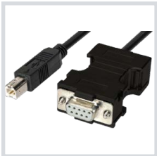
Smart Serial to USB Cable SER2-USB
