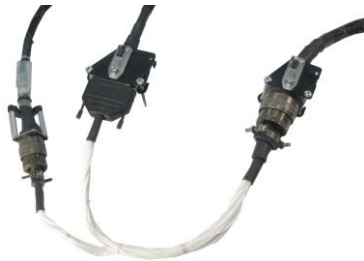
Small harness being tested with Smart-Adapters.
