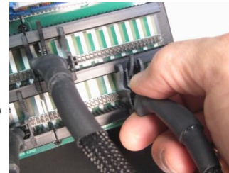
9 pin D-Sub adapter cable
