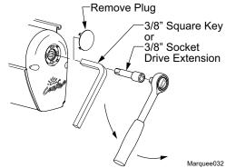
Turn the handle counterclockwise until the awning is retracted.
