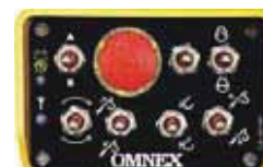
7 switch - 14 digital outputs + optional proportional trigger
