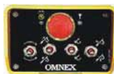
4 switch - 8 digital outputs + optional proportional trigger
