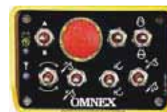
7 switch - 14 digital outputs + optional proportional dial
