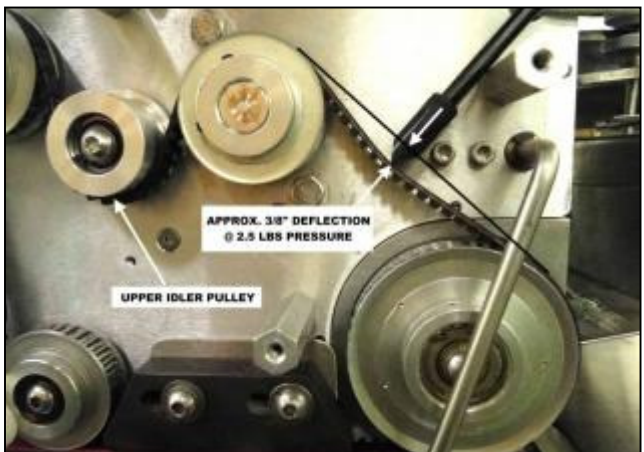
Fig. 3-7 Upper Idler Pulley
