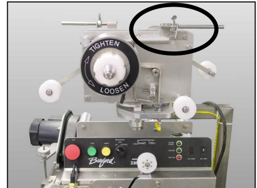
Fig. 3-13 Setting Brake Tension
