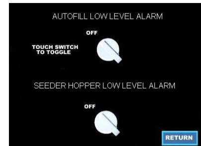
Fig. 3-7 Level Alarms Screen
