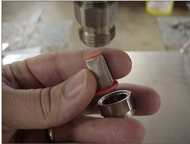
Fig. 5-1 Check Screen Replacement
