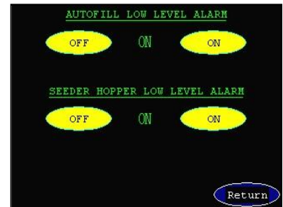
Fig. 3-8 Level Alarm Screen
