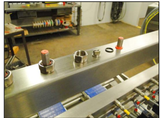
Fig. 5-1 Spray Valve Assembly
