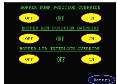
Fig. 3-17 Hopper Override Screen
