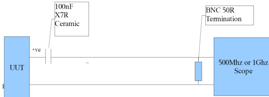
Figure 14-1 Setup for noise measurement
