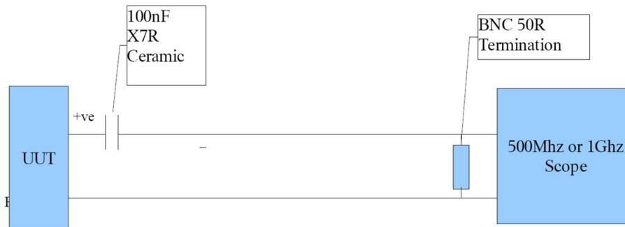
Figure 14-1 Setup for noise measurement
