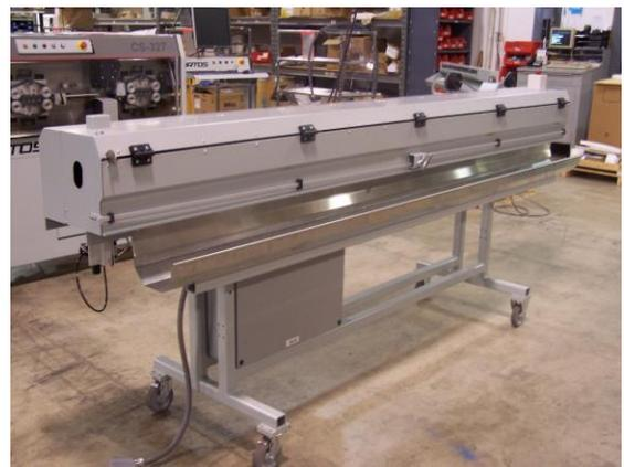
The out feed guide is removed from the **CS327** and the **CD-16** guide is positioned in its place to receive the wire from the outfeed system.
