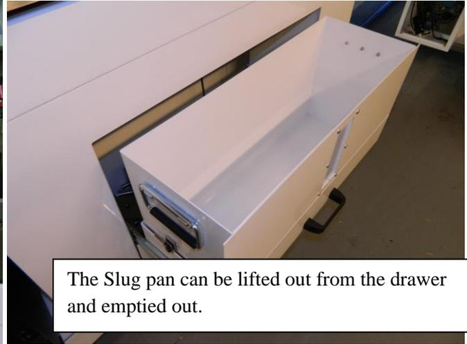
The Slug pan can be lifted out from the drawer and emptied out.
