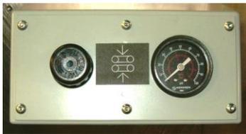
The feed belt tension is set via the regulator on the front panel. 40 to 60 PSI is a nominal pressure to start with. The general rule is to use the min pressure need to do the job. Excessive pressure or insufficient pressure will accelerate belt wear.
