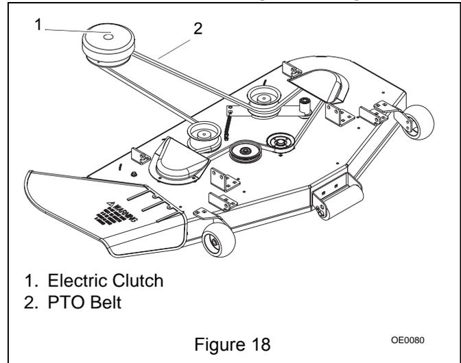
To determine if the PTO stops the mower blades within 5 seconds or less, measure the amount of time from when the PTO is shut off to when the PTO belt stops rotating.
