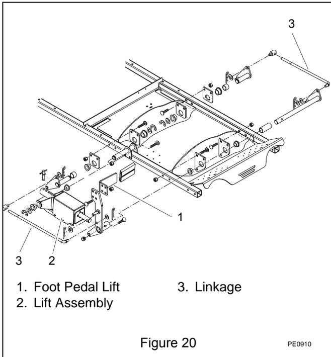
Lower deck onto blocks to remove weight from lift system.
