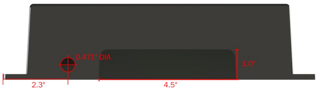
Recessed mount dimensions shown above. Mount with #6 screw.
