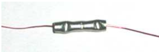
Fig. 4.3. Joining 0.0045-in.diameter wires with a crimp connector.
