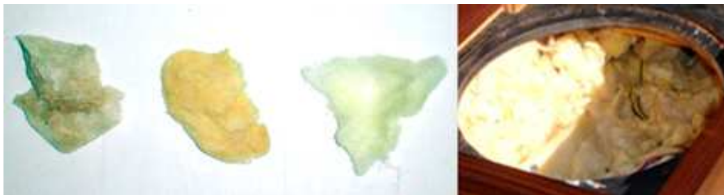
Fig. 4.4. Left: Rock wool; Center: Vintage fiberglass; Right: Modern fiberglass.
