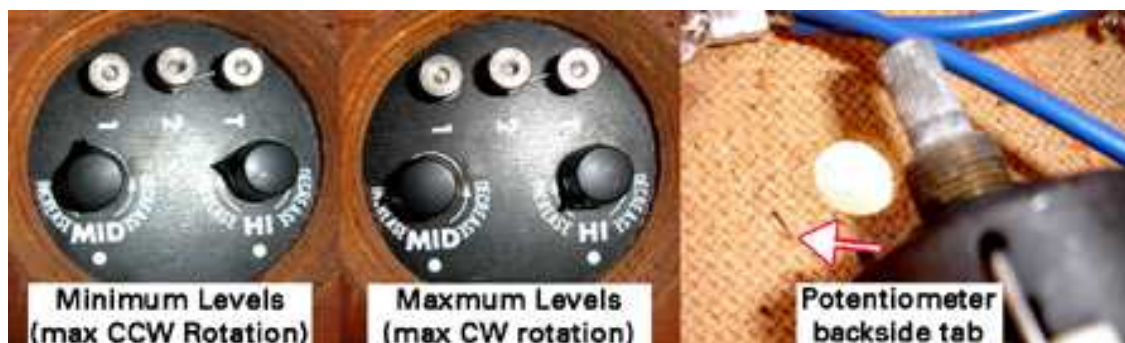
Fig. 3.14. Correct mounting of the mid-range and hi-range level control potentiometers.
