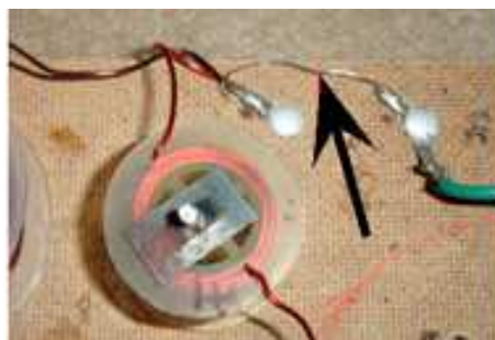
Fig. 3.7. Nichrome resistor used in early AR-3a.
