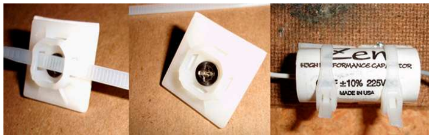
Fig. 3.18. Convenient coil and capacitor mounting bracket.
