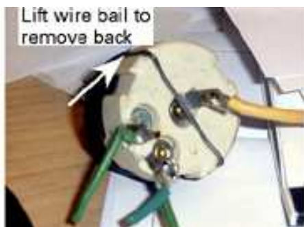
Fig. 3.11 Removing potentiometer bail
