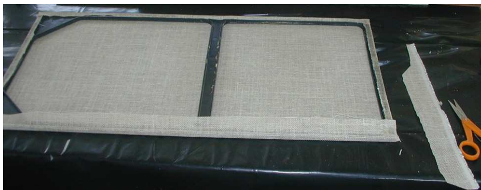
Fig. 3.20. Attaching grille cloth with gel contact cement.
