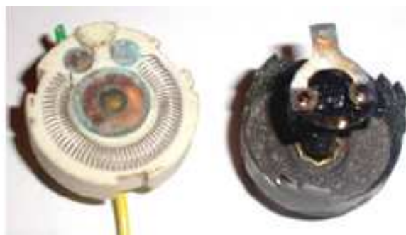
Fig. 3.12 Illustration of mild corrosion
